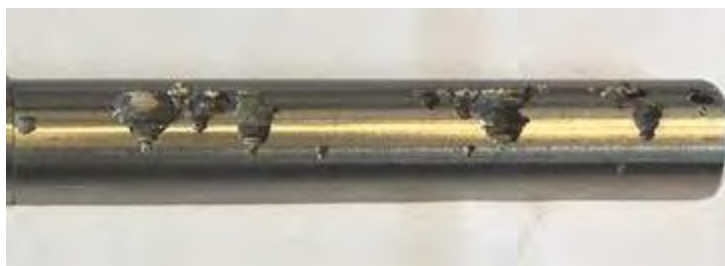
Figure 4: Sample of welded tube tested according to ASTM G48 Method C at 55 °C, after pitting corrosion took place in the surface of the sample
