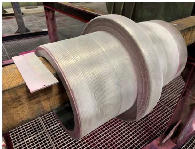
Figure 7: Mock-up overlay welding of a tube
