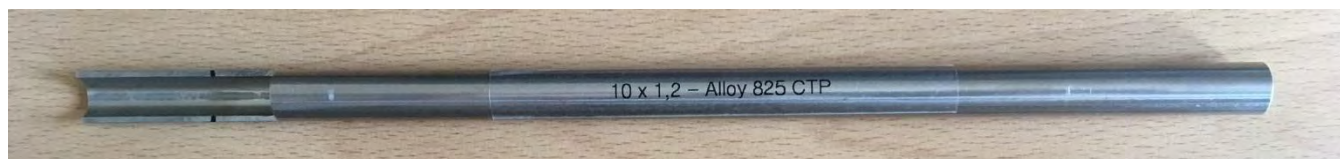
Figure 1: Autogenous plasma welded tube made of UNS N08827 plate
